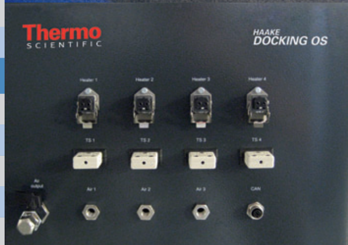
Docking Panel Connections
